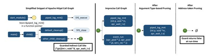
Figure 3: The effect of pruning based on argument types and taken addresses on generating a precise call graph.
